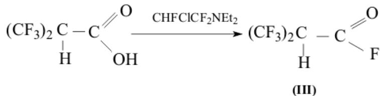
Fluoroanhydride obtained (III) was later mixed with a small excess of triethylamine while cooling and then kept in steel autoclave at room temperature. The next day methyl iodide was added to the salt obtained (IV).
